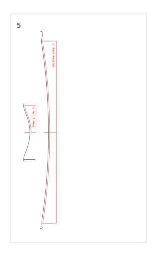
In Fig. 5. , in red, you can see the physical shape of the templates. The half templates shown here are easier done and more flexible to use than their full size counterparts.
