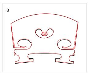
Burnish the bridge using a piece of paper with a bit of dry soap.
