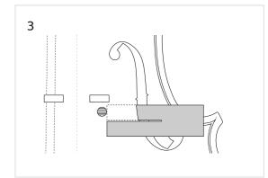
You can measure the position of the soundpost relative to the bridge foot using a simple strip of thicker paper, cut in the middle, as in Fig 3 .
