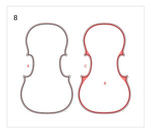
Make multiple precise passes, removing tiny shavings from the line down to the purfling. The deepest point of the fluting (and of the arching) is usually placed at the purfling or a little bit more in. The final shape of the fluting will be defined during the scraping.
